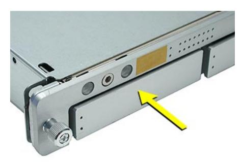
2. Grasp the drive handle, and pull the drive module out of the server. (Figure 4)
